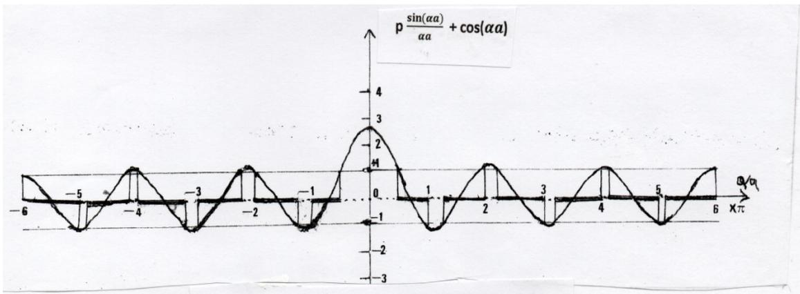
Fig.2. a Plot of the function :  $p \frac{\sin(\alpha\alpha)}{\alpha\alpha} + \cos(\alpha\alpha)$  , for  $p = \frac{\pi}{2}$
