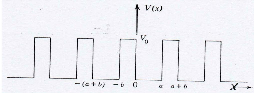
**Fig.1 : Kronig and Penney one dimensional periodic potential.**
