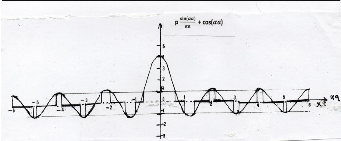
Fig.2. b Plot of the function :  $p \frac{\sin(\alpha\alpha)}{\alpha\alpha} + \cos(\alpha\alpha)$  , for  $p = \pi$
