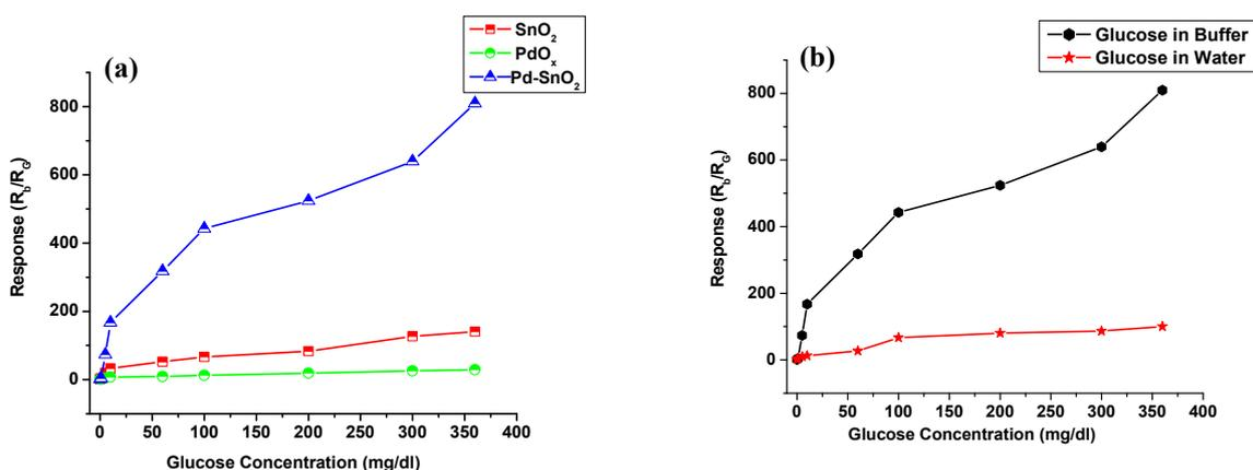
Fig 3:(a) Sensor response versus variation of glucose concentration in buffer for Pd-SnO<sub>2</sub>, SnO<sub>2</sub> and PdO<sub>x</sub> films. (b) Response versus concentration graph of glucose in buffer and water for Pd-SnO<sub>2</sub> film
