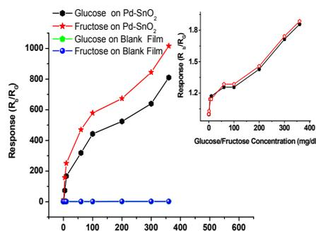
**Figure 5:** (a) Schematic diagram of films with no film deposited on the middle of the film. (b) Comparison graph of glucose and fructose response for Pd-SnO<sub>2</sub> with and without active material. Inset: Response versus glucose concentration of Pd-SnO<sub>2</sub>- film with no active material.
