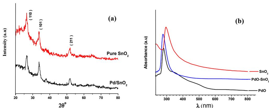
**Figure 1: (a) X-ray diffractogram and (b) UV-Vis of single step thermal decomposition nano-particle SnO<sub>2</sub> and Pd/SnO<sub>2</sub> film deposited on glass substrate.**
