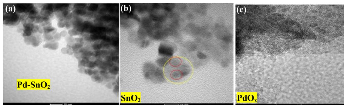
**Figure 2: TEM of (a) Pd-SnO<sub>2</sub> (b) pristine SnO<sub>2</sub> and (c) pristine PdO<sub>x</sub> deposited on glass substrate**
