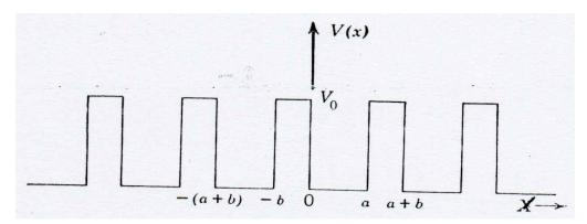
Fig.1: Kronig and Penney one dimensional periodic potential.
